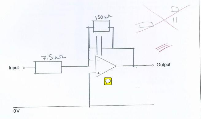
(ii) Which of these capacitors offers a break frequency closest to  $10\,\text{kHz}$ ? (Justify your choice with a calculation.) [2]  $0.1\,\text{nF} = 0.47\,\text{nF} = 1\,\text{nF} = 2\,\text{nF} = 4.7\,\text{nF} = 10\,\text{nF}$   $1 = 2\,\text{nF} = 2\,\text{nF$
