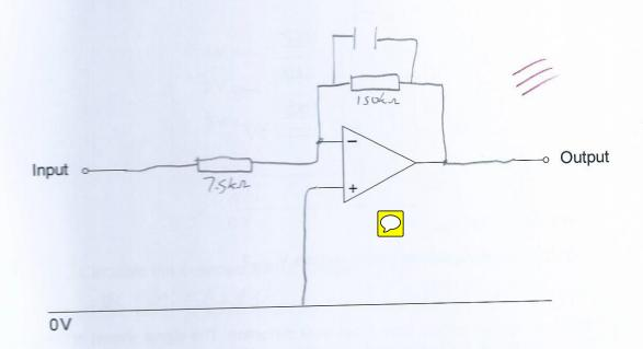
Which of these capacitors offers a break frequency closest to 10 kHz? (Justify your choice with a calculation.)
