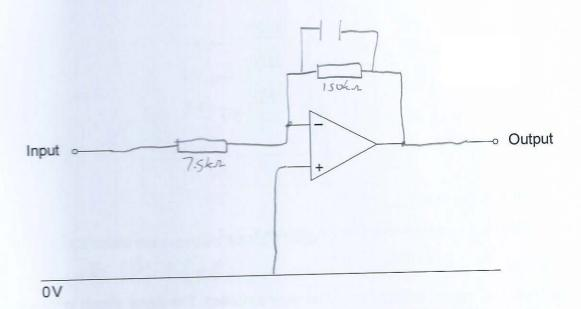
Which of these capacitors offers a break frequency closest to 10 kHz? (Justify your choice with a calculation.)
